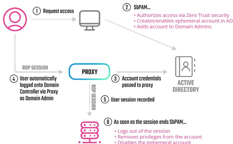
As a tier-1 component, the proxy has been designed with self-healing redundancy and the capability to scale using an architecture supported on both Windows and Linux.
